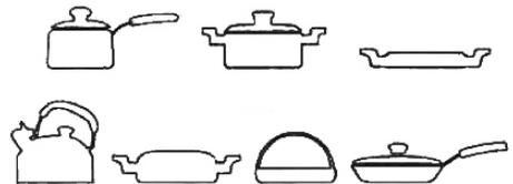
**For proper functioning, all pots and pans must have a plane magnetic bottom (a magnet must stick to it).**
